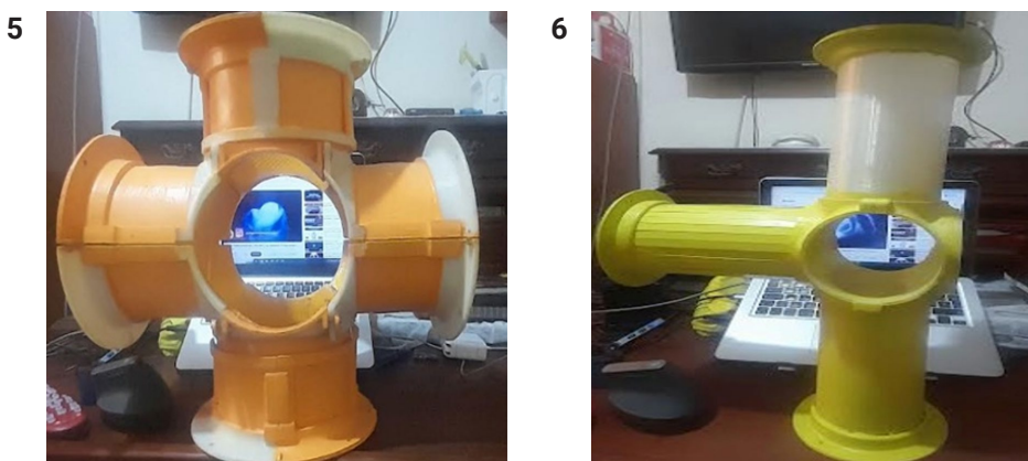
Figure 6. 5. Cross or 90-degree branch with a 6" diameter, requiring the robot to change its total position by 90° upward, downward, left, or right, or to continue forward without changing the angle. 6. Branch similar to the previous one, with a 4" diameter and a weldable connector flange [36].
