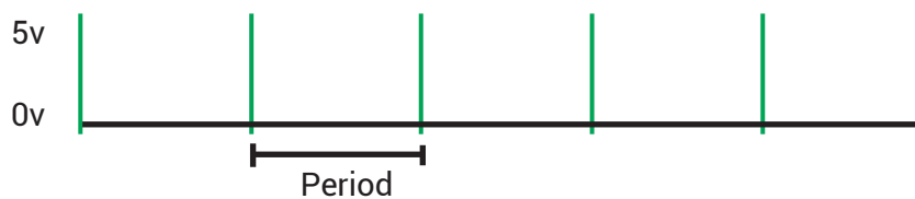
Figure 17. PWM signal with useful cycle of 0 %
